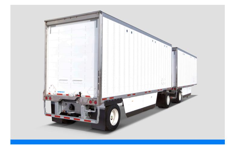
By design, Wabash Pup and Double Vans with DuraPlate Technology reduce total cost of ownership in demanding, less-than-truckload applications. With superior damage resistance, high strength for load securement and optional decking systems, our pup delivers exceptional operational value.
